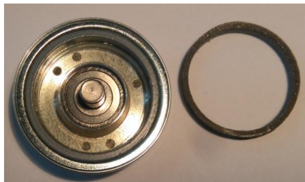
Fig.3. Results of experiment: rotor of SM motor with original permanent magnet and (on right side) magnet produced in the filament technology.
