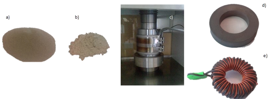
Fig.1. The material under study at different stages of preparation: a) raw Fe powder, b) PVC-S, c) the hydraulic press with a heating band used during material processing, d) the ready-made core, e) the assembled core with windings
