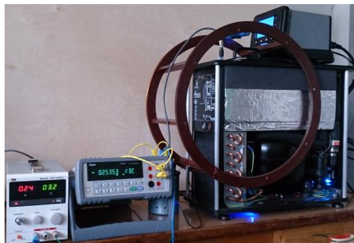
Fig.1. Developed measurement stand for investigation the temperature influence on the magnetometers
